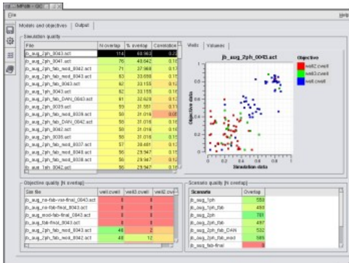
Correlation results: simulation results ranked according to goodness-of-fit with three wells
